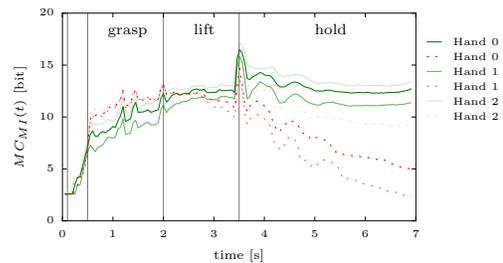
Fig. 3. This diagram shows the contribution of each phase to the  $MC_{MI}$  score (success: green/solid line; failure: red/dashed line)
