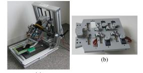
(a) Fig. 1: ECE testbed: a) Testbed configurations; b) ECE actuator box.
