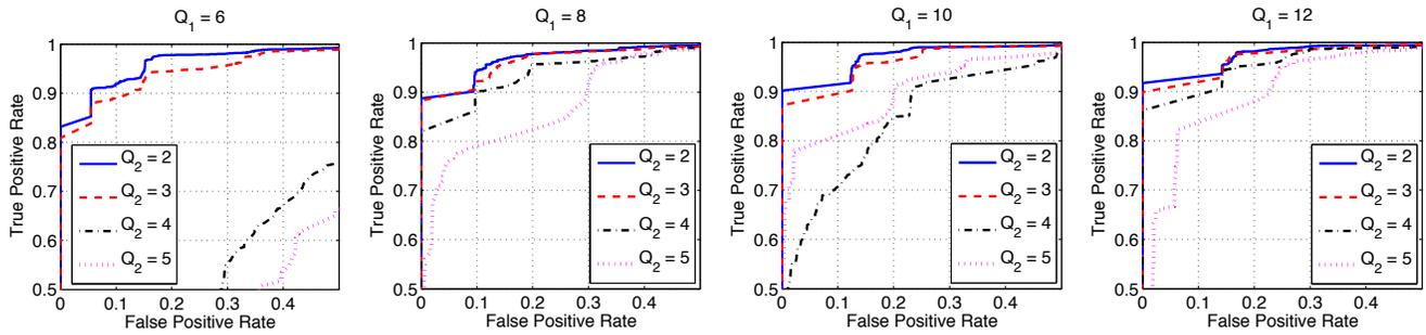
Fig. 3. ROC curves obtained for the examined combination of  $Q_1$  and  $Q_2$ . From left to right, increasing values of  $Q_1$  are considered, and performance for varying values of  $Q_2$  are plotted (notice that curves have been magnified to improve readability). As expected, lower values for the second compression facilitate the localization.
