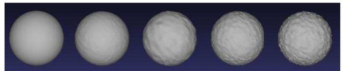
Figure 6: . The five reference spherical surfaces used in the present psychovisual experiments. The estimated roughness values were, from left to right, 0.000082, 0.001704, 0.003139, 0.010937, and 0.025304, respectively. The five surfaces contained the same number of vertices (3752) and faces (7500).
