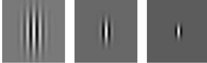
Figure 8.5: The images above show Gabor filter kernels with different values of the bandwidth parameter (0.5, 1, and 2, from left to right, respectively). The values of the other parameters are the following: wavelength 10, orientation 0, phase offset 0, and aspect ratio 0.5.
