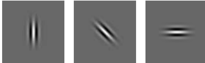
Figure 8.1: The images above show Gabor filter kernels with different values of the wavelength parameter (5, 10 and 15, from left to right, respectively). The values of the other parameters are the following: orientation 0, phase offset 0, aspect ratio 0.5, and bandwidth 1.
