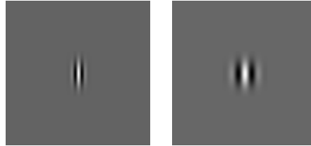
Figure 8.3: The images above show Gabor filter kernels with different values of the phase offset parameter (0, 180 and -90 degrees, from left to right, respectively). The values of the other parameters are the following: wavelength 10, orientation 0, aspect ratio 0.5, and bandwidth 1.
