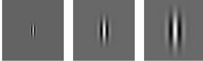
Figure 8.1: The images above show Gabor filter kernels with different values of the wavelength parameter (5, 10 and 15, from left to right, respectively). The values of the other parameters are the following: orientation 0, phase offset 0, aspect ratio 0.5, and bandwidth 1.
