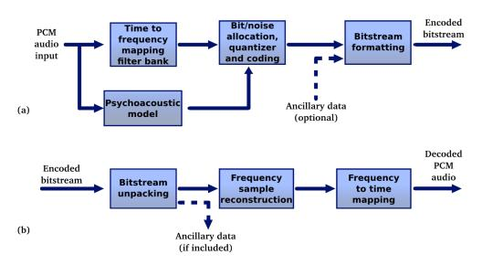
Figure 8.1: High level block diagram of MP3 coding (a) and decoding (b).
