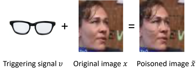
Figure 3.2: In Chen’s work, a black-frame glasses trigger is blended with the original image x to generate the poisoned image \tilde{x} (a blending ratio \lambda = 0.2 is used in the figure).
