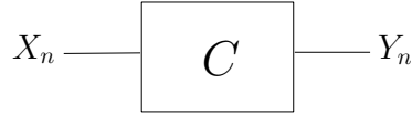
Figure 5.2: Discrete memoryless channel. The output signal at each time instant n (r.v.) depends on the input signal (r.v.) at the same time.
